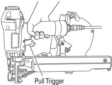
**CONTACT ACTUATION MECHANISM**
