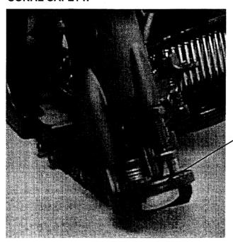
Insure Push Lever Assembly is free to travel up and down. Clean and lubricate Push Lever Assembly and washer feed path before each day of use with a silicone spray lubricant for optimal performance.
