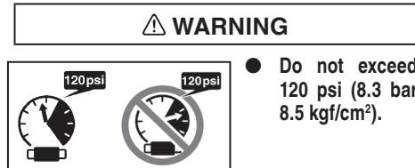
Adjust the air pressure at recommended operating pressure 70 – 120 psi (4.9 – 8.3 bar 5 – 8.5 kgf/cm<sup>2</sup>) according to the length of nails and the hardness of workpiece.
