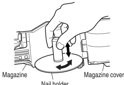
**NOTE:** Before loading nails in the magazine, adjust the plate. If the magazine cover is forcibly closed without adjusting the plate correctly, the nail holder may be damaged.
