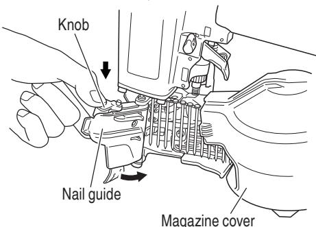
**NOTE:** Be careful not to deform the collated wires and not to disengage the nails with the guide surface. Otherwise, the nail guide will not close correctly.
