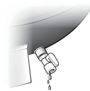
Drain valve (open)
