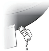
Drain valve (open)
